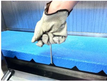
To lift the dog wash floor, open the dog entry door, using the tool as shown above, slide the hooked end under the front edge of the floor and slide sideways until the hooked end locates into one of the notches in the front edge, then lift.
