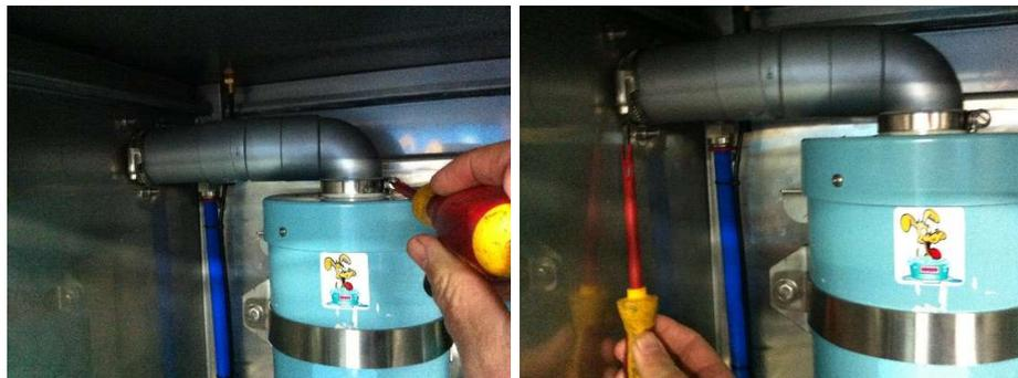
Please note heated dryers only have the one clamp but have a screw that needs to be tightened.
