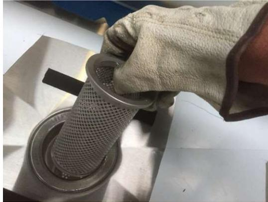
While the filter is removed, place the wash gun in the drain, set the wash gun to “JET”, rotary dial selection to RINSE and flush the drain. Run the water gun for 20 seconds, if there are issues with the water draining away you may need to contact your plumber. Replace the cylindrical filter, and put the stainless-steel filter back into position.
